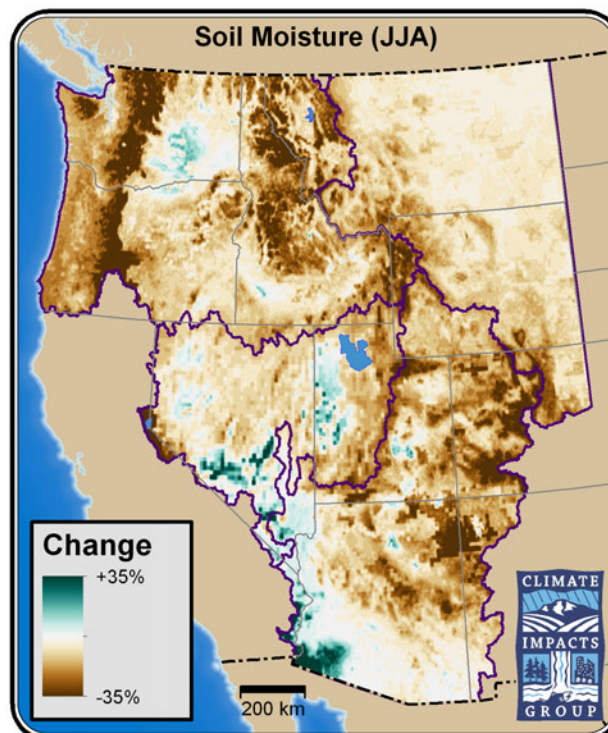
Figure 20: Projected change in total soil column moisture, in percent relative to historical (1916-2006), for the 2040s for a moderate warming scenario (A1B) using the Miroc 3.2 and PCM1 global climate models and the VIC hydrologic model. 32
